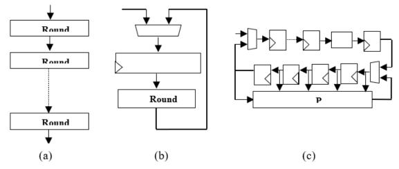
Figure 2. Basic Implementation Methods (4-a) unrolled, (4-b) round and (4-c) serial implementation
