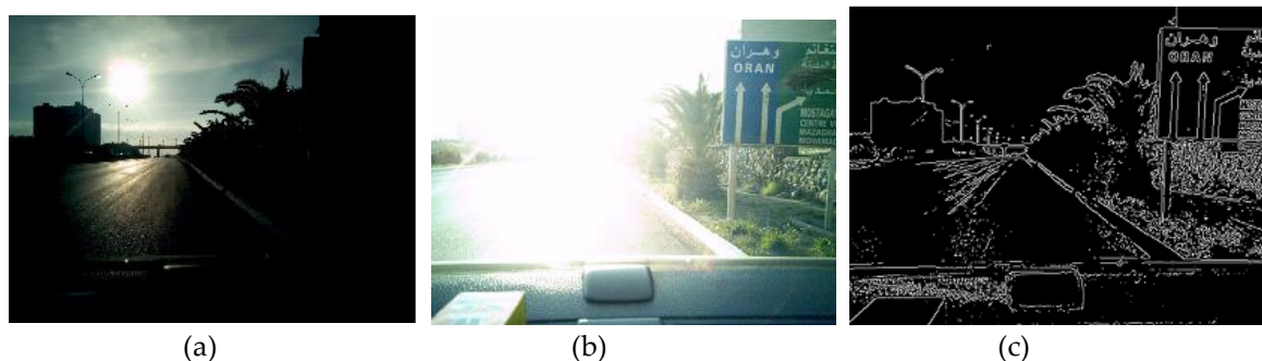
Figure 1. Exposure Fusion Neural Network facing High Dynamic Range Scene: (a) Auto exposed image; (b) Saturated image; (c) Exposure Fusion + Canny Edge Detection.
